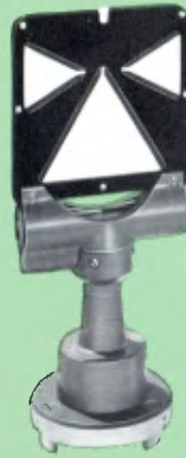
Target of traverse equipment with tribrach of T2
