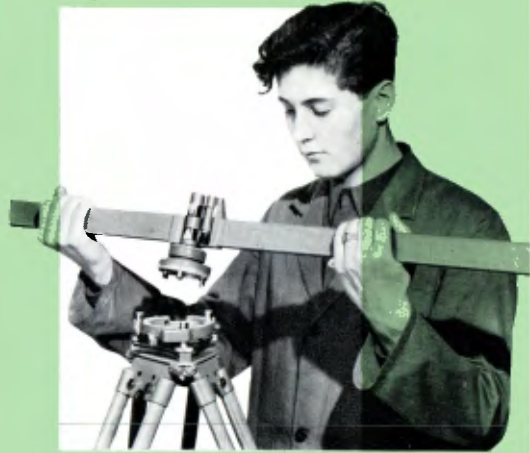
Mounting the invar subtense bar on the tribrach
